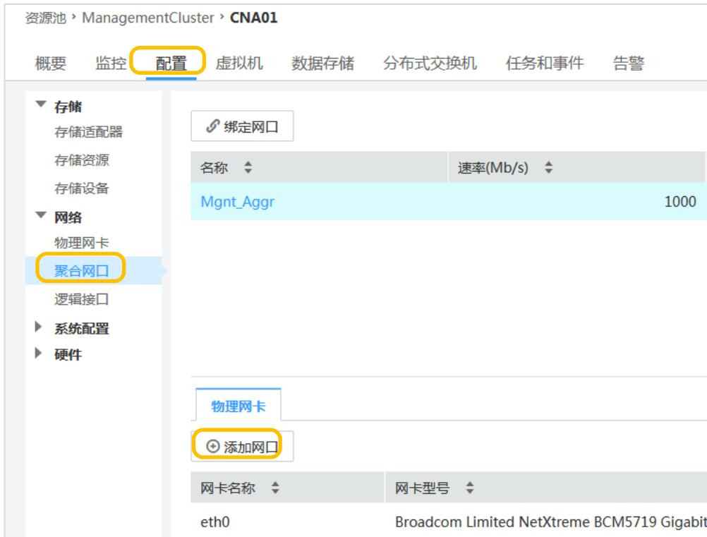
The screenshot shows the host configuration page for 'CNA01'. The 'Configuration' tab is selected. In the left sidebar, '聚合网口' is highlighted with a yellow box. Below it, there's a table for 'Mgnt\_Aggr' with a rate of 1000 Mb/s. At the bottom, there's a '物理网卡' section with a '添加网口' button highlighted with a yellow box. The table below shows 'eth0' with the model 'Broadcom Limited NetXtreme BCM5719 Gigabit'.
